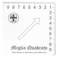
In this example locate the intersection of the 33 and 81 grid lines. Position the romer so that its upper right corner is at the intersection (and it is aligned with the upper edge along the 81 line).
